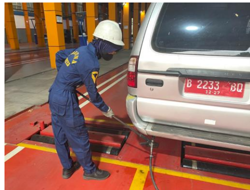
Gambar IV. 11 Pengujian Smoke Tester
