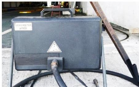
**Gambar III. 3** Alat Uji Smoke Tester
