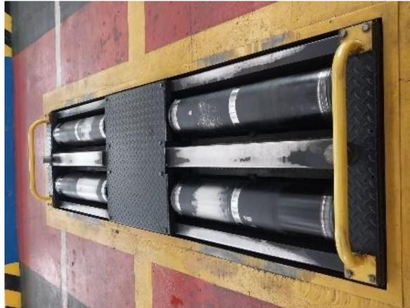
**Gambar III 9** Speedometer Tester
