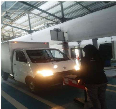
**Gambar IV. 8** Pengujian Headlight Tester
