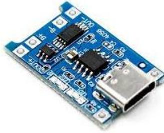
**Gambar III. 14** Module Charger TP4056(Ariawan, 2020)
