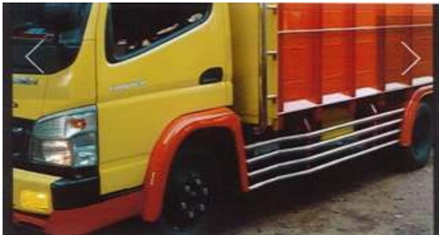
**Gambar 2. 22** Perisai Kolong Samping Pipa Besi
