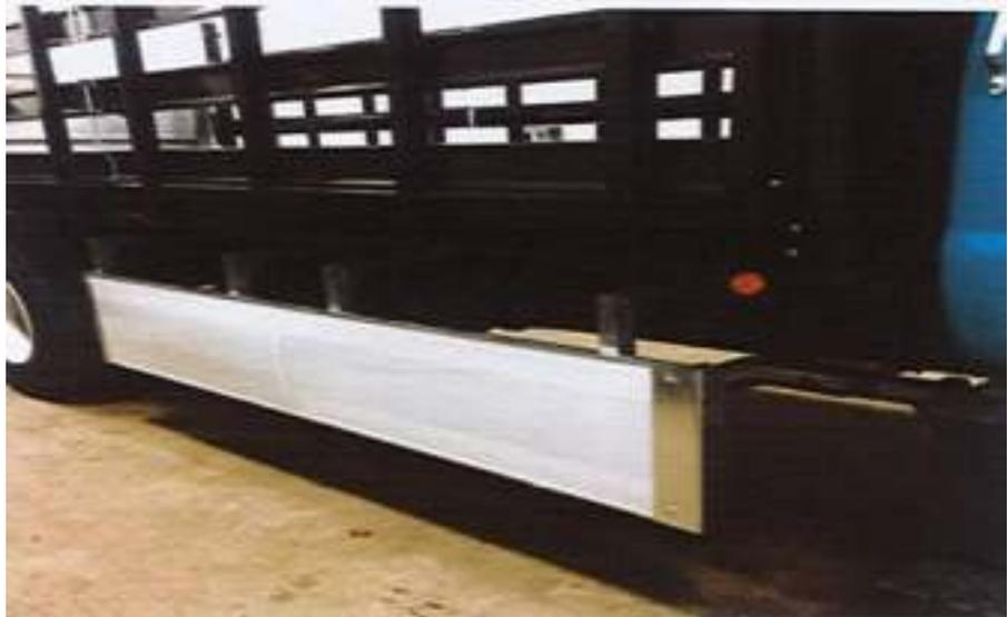
**Gambar 2. 23** Perisai Kolong Samping Plat Besi / Fiber
